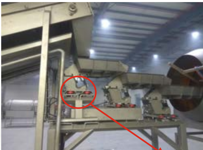
Rubber Mounting isolate vibration in Dynamic Weigher Machine
