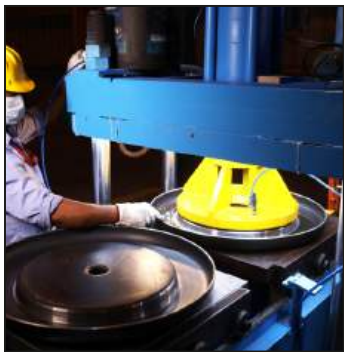
WELD AIR TIGHT TEST
