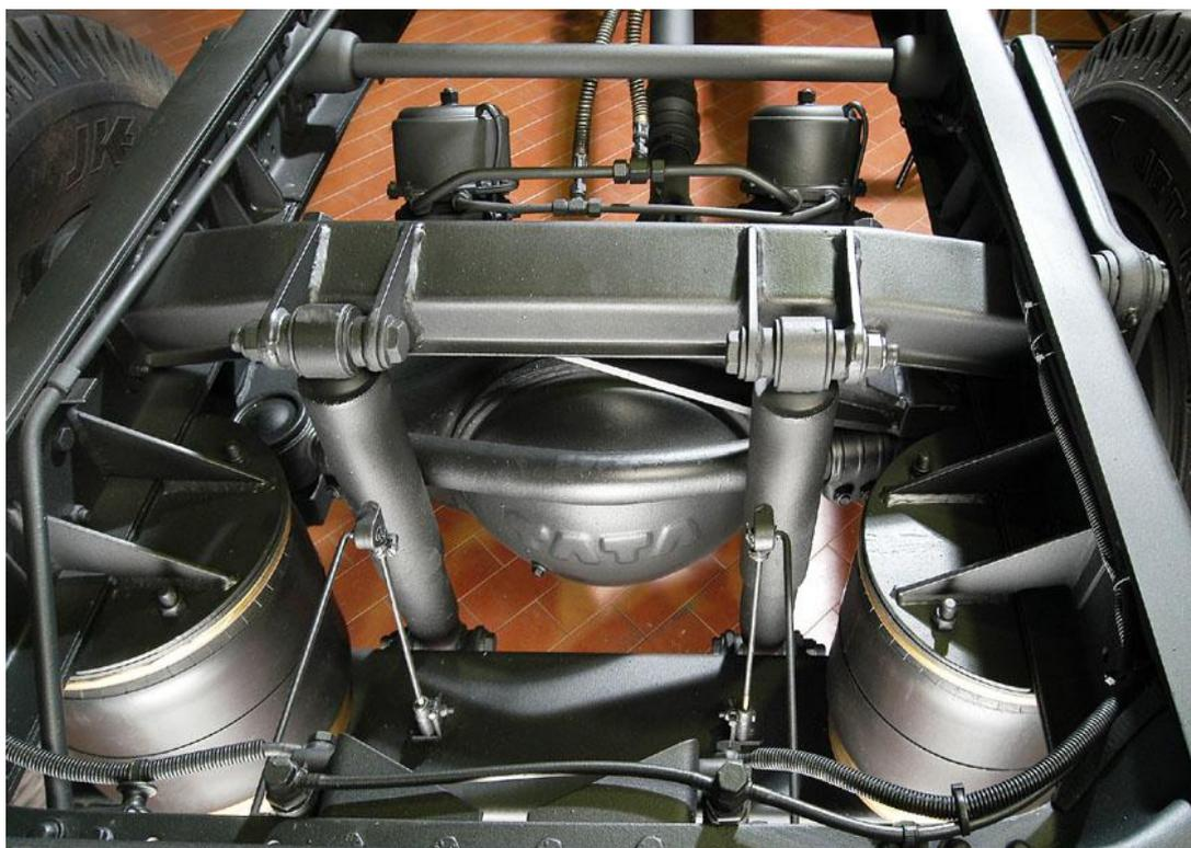
The conventional leaf springs (L.S.) in the Suspension System of a Vehicle has a load / deflection Curve which has a constant slope. But, with very low available travels and static deflections as also high hysteresis, there are obvious constraints with regard to achieving comfort levels inside the vehicle. In spite of shock absorbers used in "Tandem" the leaves of the bundled spring are subject to fatigue as well as impact stresses due to which vibrations and shock are routinely experienced.
